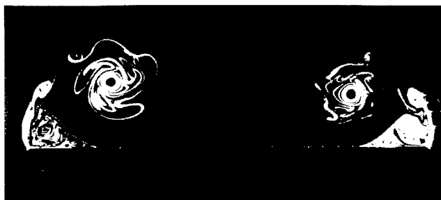
Fig. 2 Smoke flow visualization of vortex over a 70-deg sweep delta wing at 20-deg angle of attack. 8
